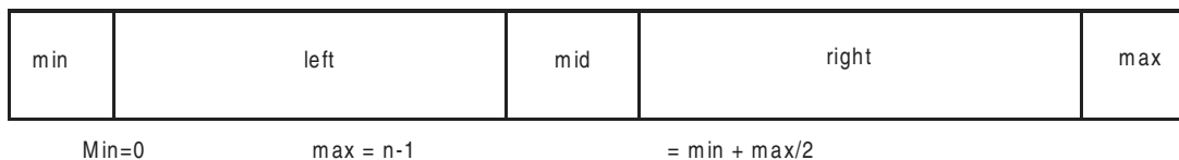
Fig. 14.2a Binary search technique. Original array
